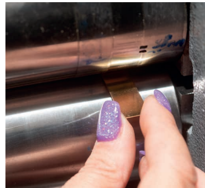
Fig 5 - Hand feeding a piece into rollers - tapering
